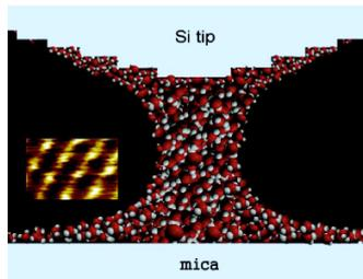
FIG. 1. Experimental schematics of a high sensitivity AFM setup operating in ambient conditions. The inset shows an atomic-resolution AFM image of a dry and clean mica substrate, obtained at a modulation-amplitude change of 5% (scan area: 1.5nm×1nm) [3].
