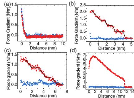
FIG. 2. Measured values of the force gradient of the water meniscus as a function of its elongation at a given RH of (a) 2%, (b) 15%, (c) 31%, and (d) 45%. The approach and retraction speed is 0.15 nm/s. The black solid line in (b) and (c) is a guide to the eye.
