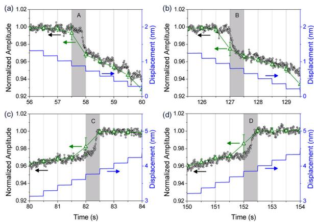
FIG. 1. The normalized amplitude measured during formation (a,b) and rupture (c,d) of the nanoscale water bridge. The gray-painted parts of (a) and (c) show a time lag of the change in amplitude, whereas there is no time lag in (b) and (d).
